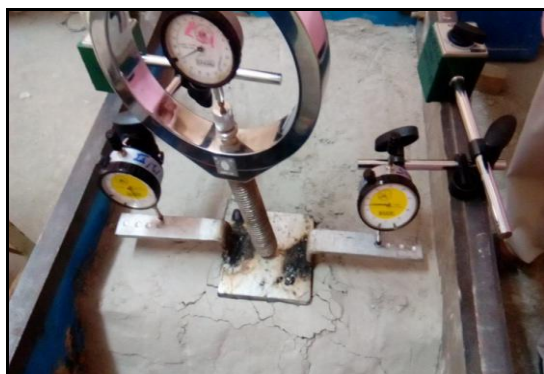
Figure 3.2.4 Failure of slope
